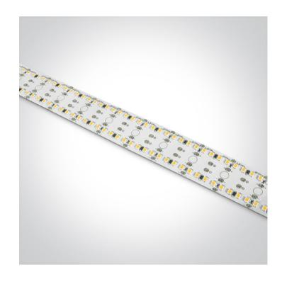
Flexible LED light strip, with SMD2835 LEDs, 33W/meter. Supplied in 5 meters roll with white PCB and double adhesive tape for a better fixing.
